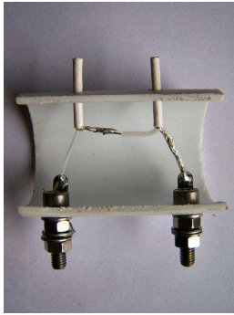
PHOTO.1 Series connection of the inner and outer to provide high inductance and low capacitance.
