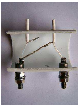
PHOTO.2 Parallel connection, with the inner of the coax as the inductance, to provide low inductance and high capacitance.
