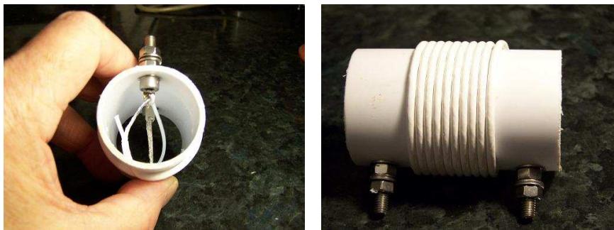
PHOTO 4 & PHOTO 5 show a complete 40 meter trap.
